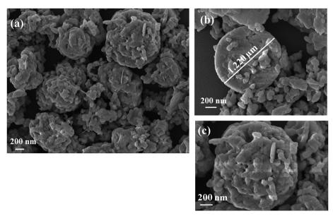
Fig. 2. FEG-SEM micrographs of  $ZnMoO_4$ :  $Tb^{3+}$ ,  $Pr^{3+}$  particles prepared by the sonochemical method,  $ZnMoO_4$ :  $ZnMOO_4$ :
