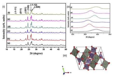
Fig. 1. X-ray diffraction of the  $ZnMoO_4$  and  $ZnMoO_4$ : $Tb^{3+}$ ,  $Pr^{3+}$  particles.
