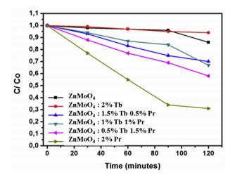
**Fig. 10.** Variation in the concentration of the methylene blue dye against the synthesized  $ZnMoO_4:Tb^{3+}$ ,  $Pr^{3+}$  powders submitted to UV radiation. (For interpretation of the references to color in this figure legend, the reader is referred to the Web version of this article.)
