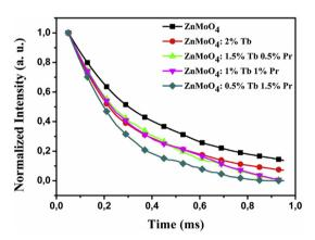
Fig. 9. The luminescence decay curves (excited at 350 nm and monitored at 545 nm) of  $ZnMoO_4:Tb^{3+}$ ,  $Pr^{3+}$  phosphors with different  $Tb^{3+}$  and  $Pr^{3+}$  codoping concentrations.
