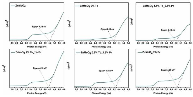
Fig. 5. Gap energy of ZnMoO<sub>4</sub> and ZnMoO<sub>4</sub>:Tb<sup>3+</sup>, Pr<sup>3+</sup> samples.
