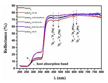
Fig. 4. Absorption spectra of the ZnMoO<sub>4</sub> and ZnMoO<sub>4</sub>: Tb<sup>3+</sup>, Pr<sup>3+</sup> samples.
