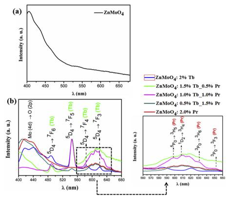
Fig. 6. Emission spectra of ZnMoO<sub>4</sub> and of ZnMoO<sub>4</sub>:Tb<sup>3+</sup>, Pr<sup>3+</sup>.
