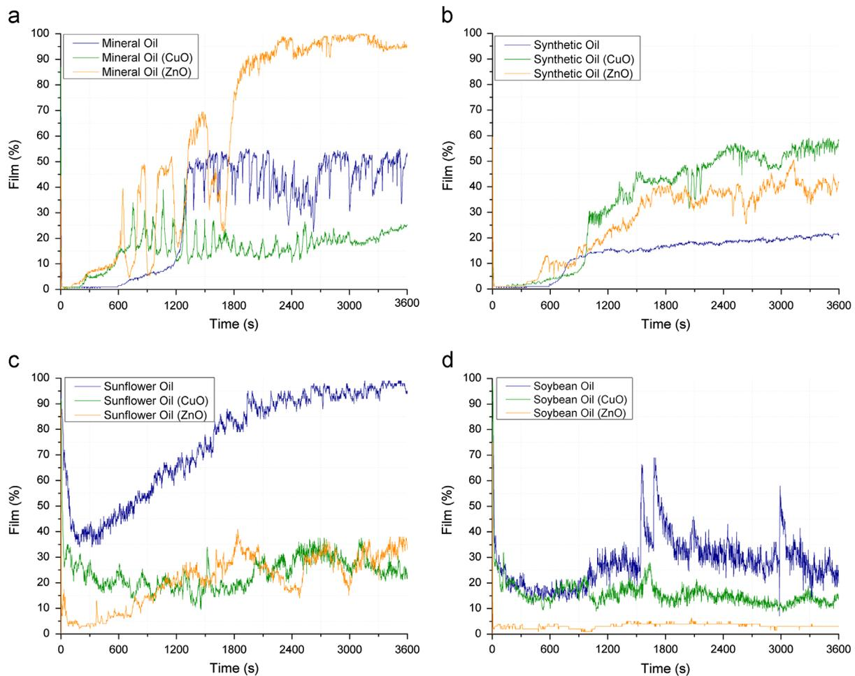
Fig. 5. Film formation as measured by ECR for all lubricant and additives tested: (a) mineral oil, (b) synthetic oil, (c) sunflower oil and (d) soybean oil.
