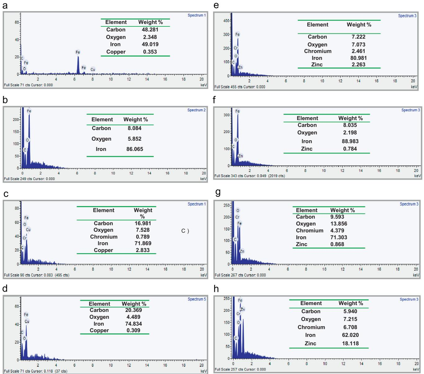
**Fig. 8.** EDS analysis of worn surface of steel disc for: (a) sunflower oil+CuO, (b) soybean oil+CuO, (c) synthetic oil+CuO, (d) mineral oil+CuO, (e) sunflower oil+ZnO, (f) soybean oil+ZnO, (g) synthetic oil+ZnO and (h) mineral oil+ZnO.
