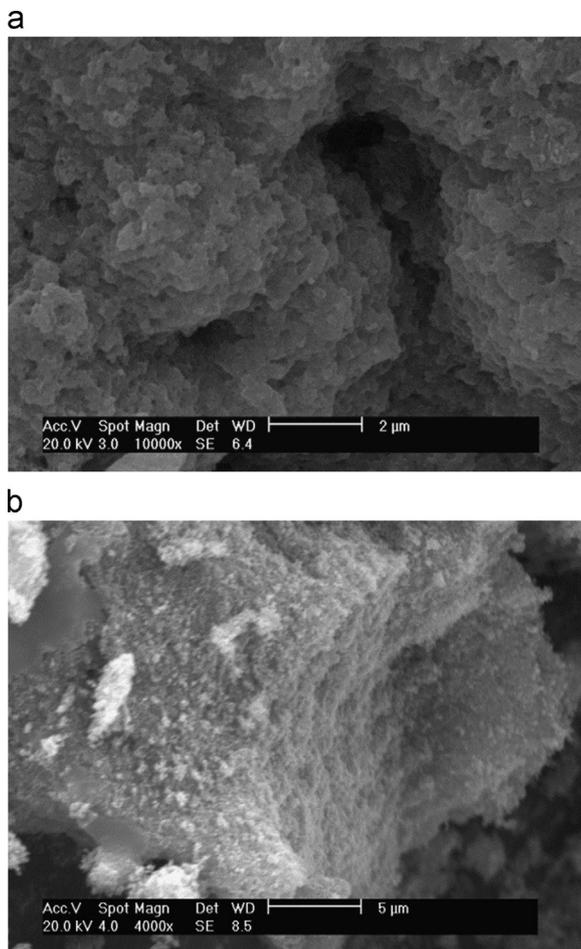
Fig. 2. SEM micrographs of the prepared samples (a) CuO and (b) ZnO.
