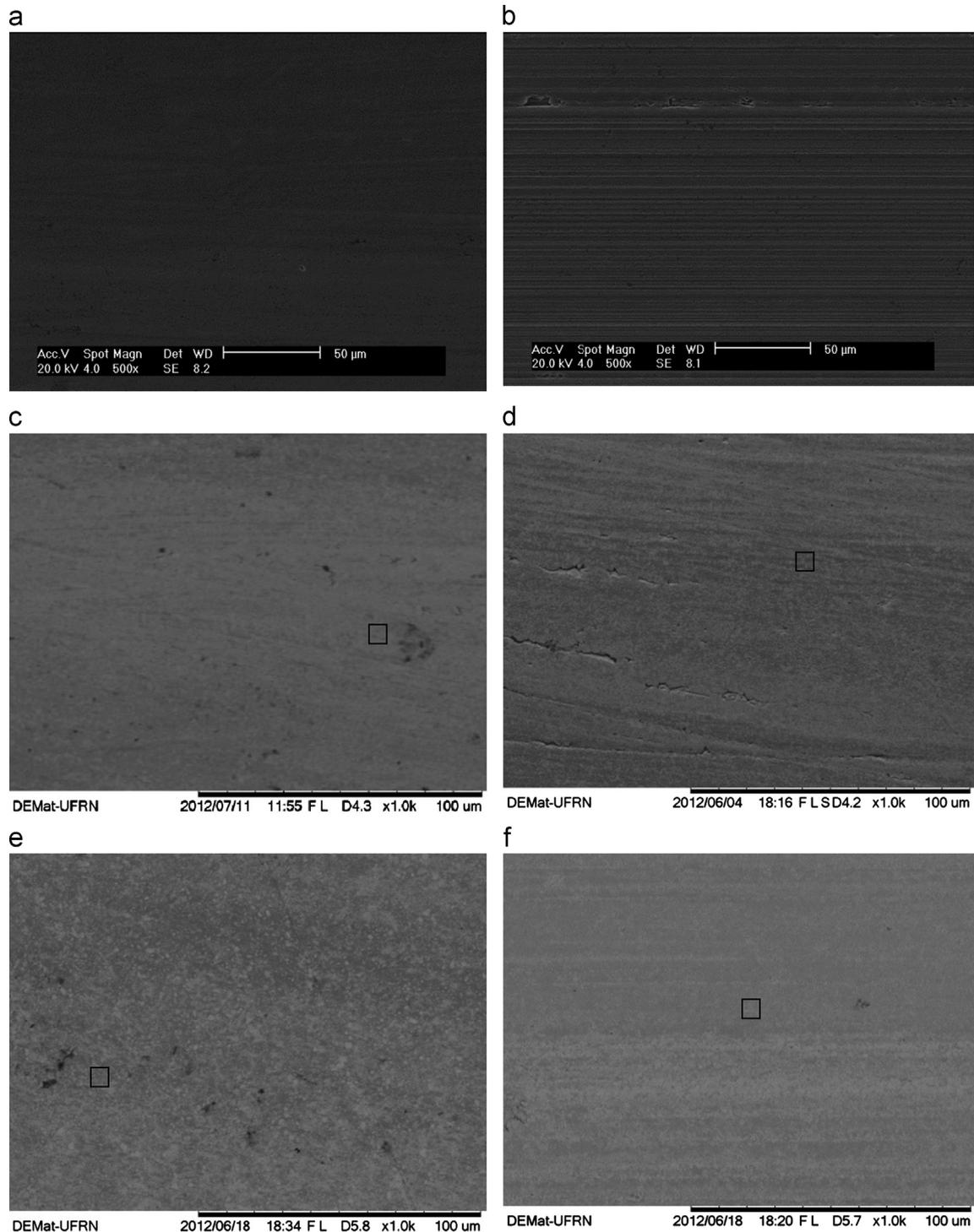
**Fig. 7.** SEM micrographs of the worn surfaces lubricated with: (a) synthetic oil (WSD =  $303.5 \pm 2.2 \mu\text{m}$ ) (b) mineral oil (WSD =  $269.5 \pm 4.9 \mu\text{m}$ ) (c) synthetic oil+CuO (WSD =  $280.2 \pm 2.5 \mu\text{m}$ ) (d) mineral oil+CuO (WSD =  $276.5 \pm 3.2 \mu\text{m}$ ) (e) synthetic oil+ZnO (WSD =  $293.0 \pm 4.5 \mu\text{m}$ ) and (f) mineral oil+ZnO (WSD =  $256.0 \pm 4.2 \mu\text{m}$ ).
