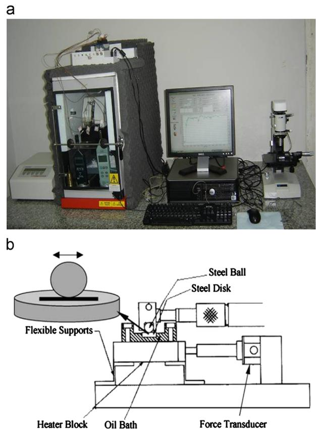
Fig. 3. HFRR test: (a) image of equipment used in tests and (b) schematic diagram of HFRR.
